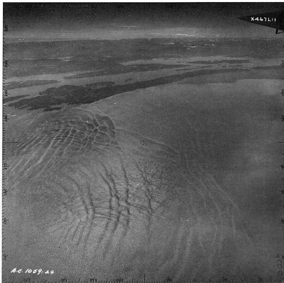
Fig. 2.3. Surface slicks produced by internal waves (British Columbia Air Photographic Service).
